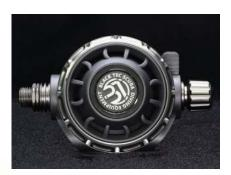
BT-8 is a Pneumatic Balanced Second Stage Regulator equipped with user adjustable knob and a Venturi switch control. The metal air barrel as well as the large heat exchange comes as standard and increase the resistance to freezing in extreme conditions. The pneumatic balanced design reduces the inhalation effort required to open the second stage valve and substantially improves the overall ease of breathing in all diving conditions,
